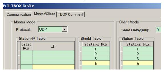
The settings of T-BOX1 and T-BOX2 in the Master mode are shown as following: (turn off DIP switch 1)
