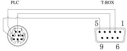
(2) When use RS-485 port, port A is "+", port B is "-", and connect port A, B with PLC port A, B.
