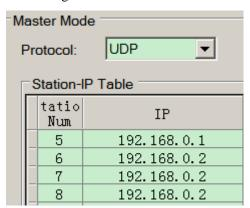
Station IP table: station NO.5, NO.6 No.7 and NO.8 are slave station numbers. IP is the slave device IP address.
