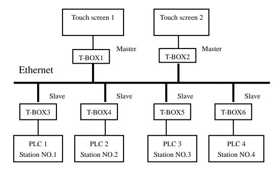
In this system, there are 6 T-boxes, T-BOX1 and T-BOX2 are master mode, others are Slave T-BOX. Touch screen 1 and touch screen 2 are master device, PLC1, PLC2, PLC3 and PLC4 are all slave devices.
