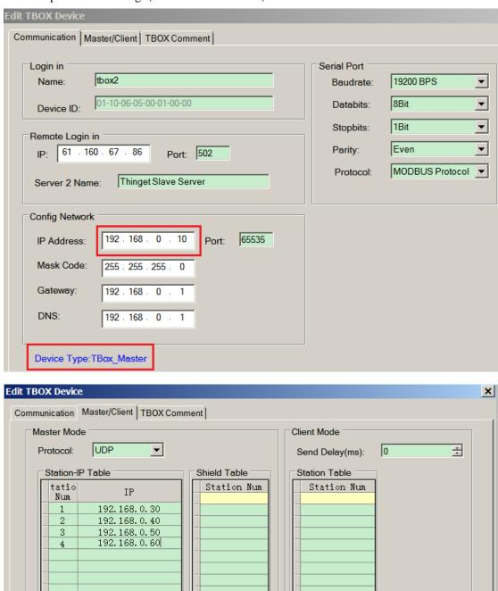
T-BOX2 parameters setting: (Turn off DIP switch 1)
