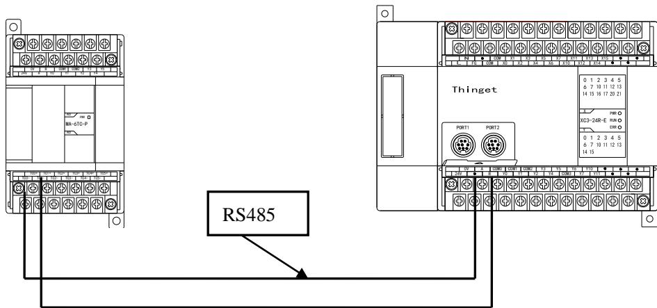
(2) Communication parameter setting: baud rate is 19200bps, module station number is 1.
