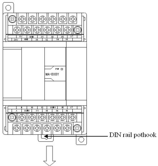
The MA modules can be installed on the DIN46277 rail ( width 35mm ). When uninstalling, pull down the pothook of the DIN rail.
