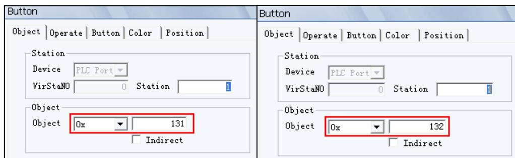
After connecting with touch screen, the user can realize reverse function for Y3 and Y4 on touch screen.
