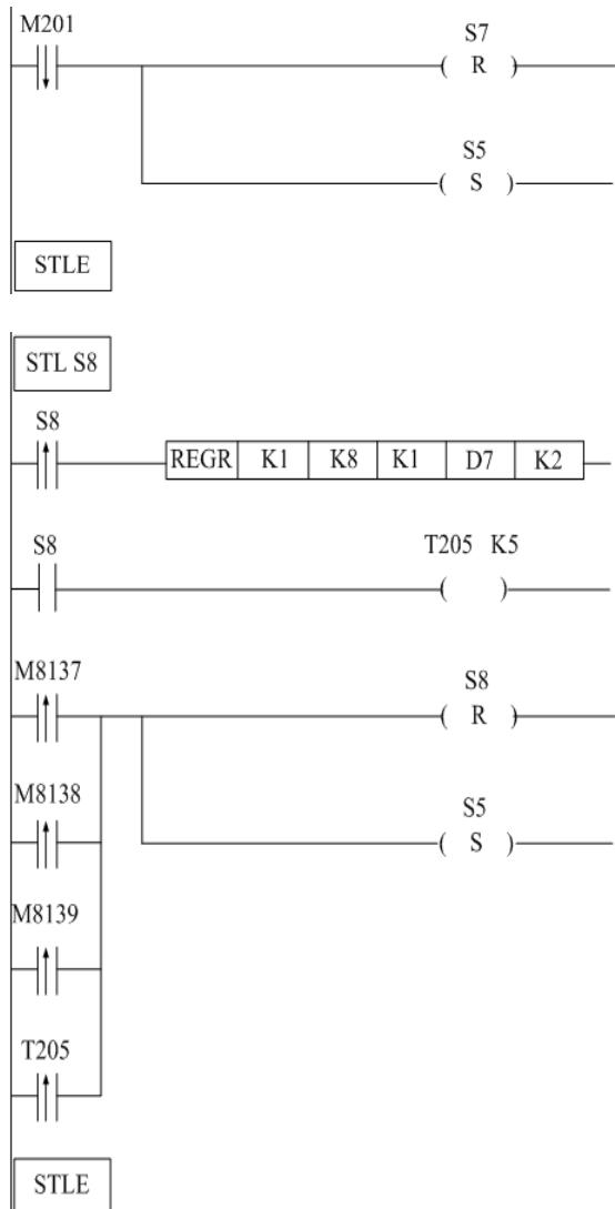
Close process S7 and open process S5 when data transfer are completed or 50ms is over
