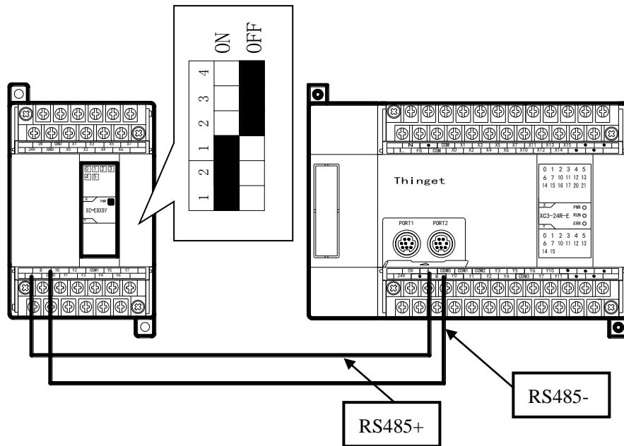
For this example, write the value of PLC coil into MA I/O points, read the value of MA I/O points to PLC coil.
