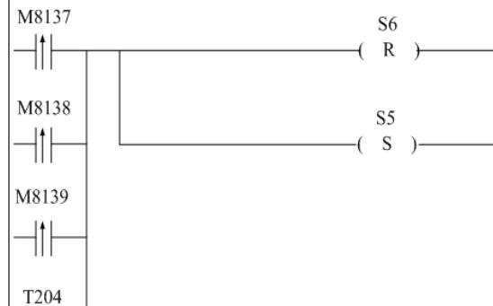
Close process S6 and open process S5 when data transfer are completed or 50ms is over
